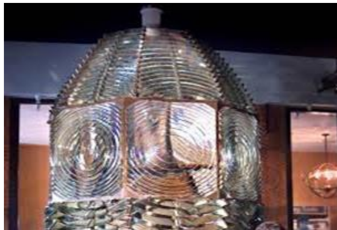
The Fresnel lens was a French invention that helped to greatly magnify a very small light source.
