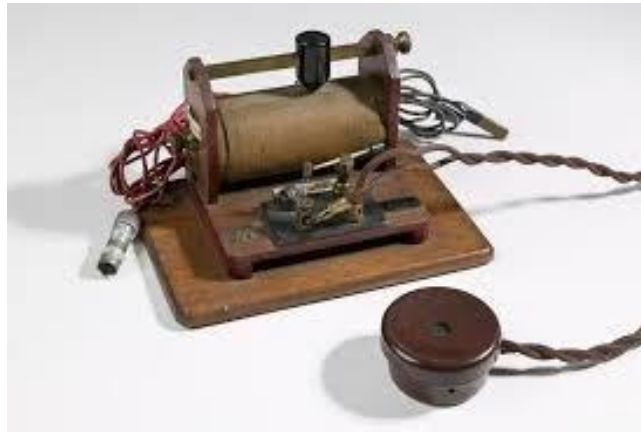
Typical basic crystal set, with one headphone
