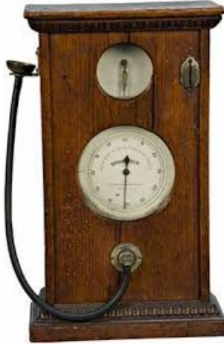
Arcade visitors would pay to blow into this machine to test their lung power. Sanitary?
