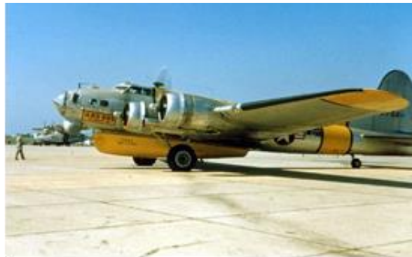
The Higgins A-1 Lifeboat is shown attached to a rescue B-17.
