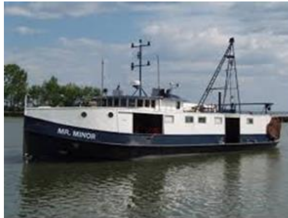
A fish tug rigged for trawling. Note the net lifting crane on the top and the sled on the rear
