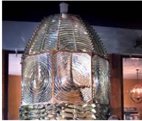
The Fresnel lens was a French invention that helped to greatly magnify a very small light source
