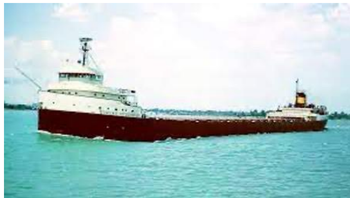
The 729-foot Edmund Fitzgerald was typical of the post-1943 MacArthur Lock ship designs that my friends sailed on. She was a classic ore boat design with her wheelhouse forward and engine aft, as well as a self-unloader.
