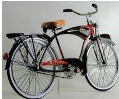
The venerable Schwinn Phantom was equipped with stock whitewall tires, headlight, spring suspension, luggage carrier, and an in-tank horn.
